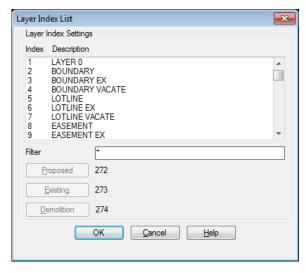
Proposed, Existing and Demolition are Layer Types. When SmartDraft creates a layer, it reads the layer database index number associated with the current layer type. To enter or select a layer database index number, it must already exist in the layer database file
